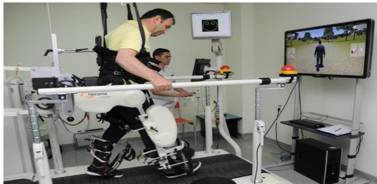
Fig. 4. Walking Robot with Suspension-Pulley System [18]
